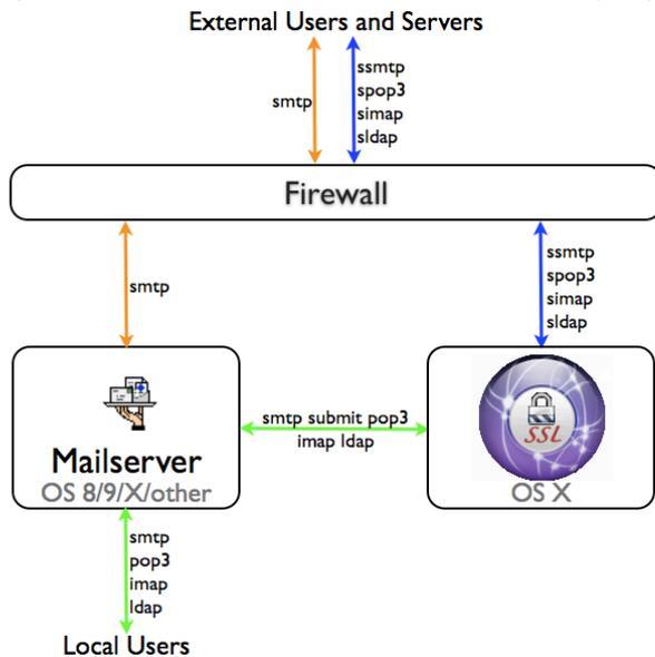
One of the extensions within mail protocols is the addition of the TLS (Transport Layer Security) encryption and authentication protocol. When a client and server that support TLS talk to each other, they can encrypt the data channel and thus guard against eavesdroppers.
